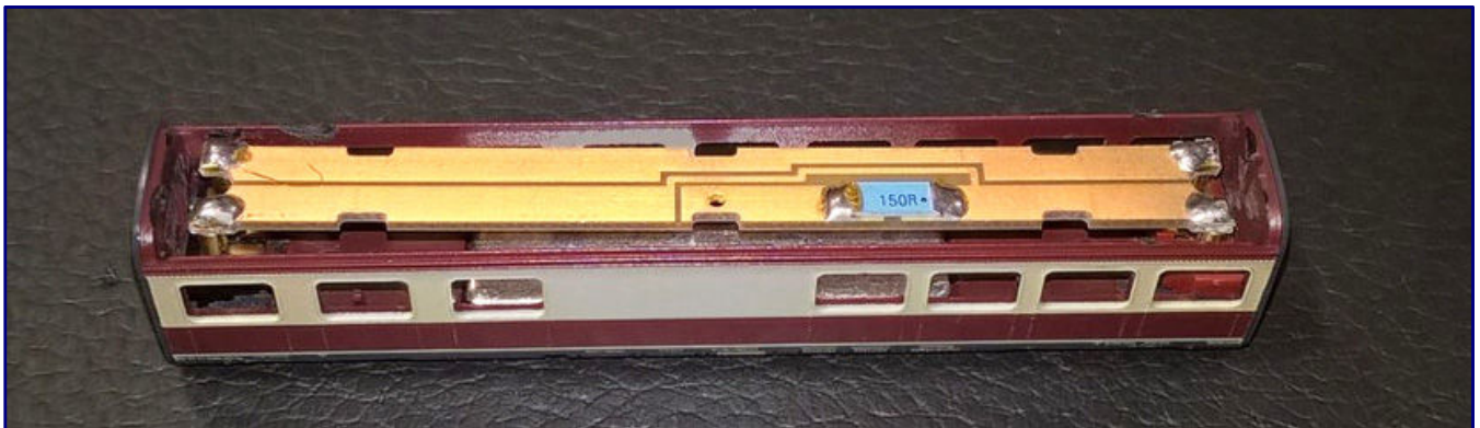
Test assembly: The board is still a little crooked, but this does not cause any problems during further assembly and subsequent operation on the layout. Photo: Torsten Scheithauer
