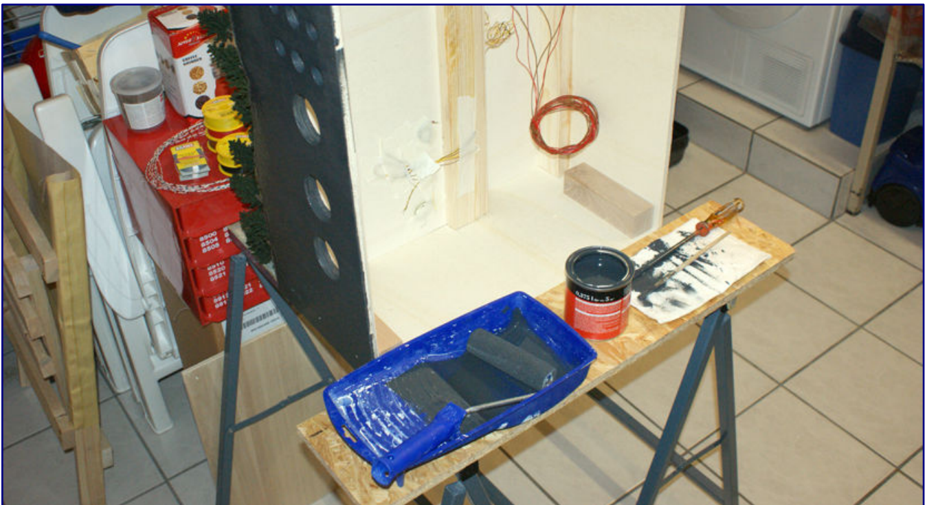
The diorama box is painted in dark grey. The paint is applied with a brush at the edges as well as at the border to the terrain transition (top), and with a paint roller for the rest of the surface (bottom).
