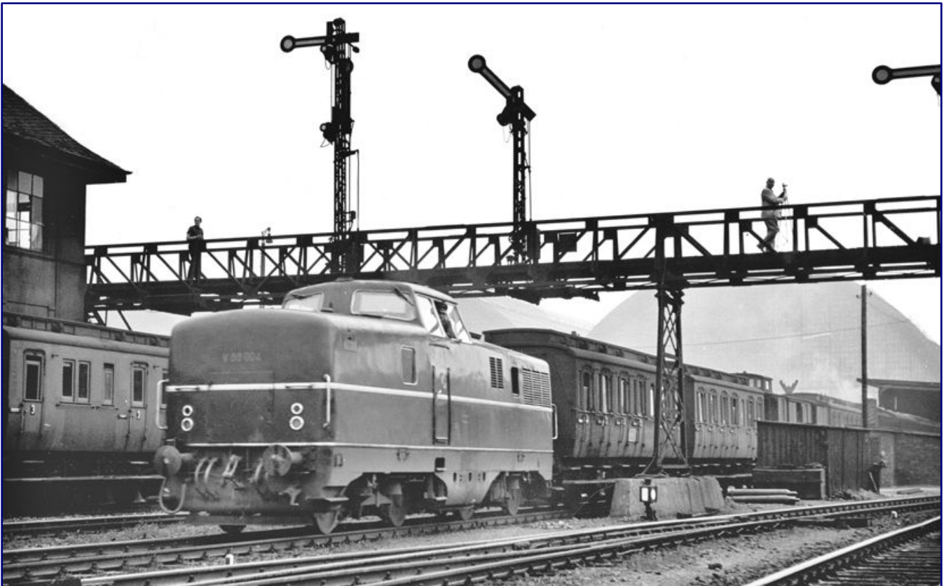
V 80 004 from the Frankfurt-Griesheim depot pushes its passenger train of blunderbusses between the Galluswarte branch and Frankfurt-West in 1954 without a doubt under indirect push-pull control, as can be seen from the direction of view of the driver remaining on the locomotive (photo above). The same locomotive still had to make do with Prussian compartment coaches when it left Frankfurt's main station in October 1952 (photo below). The three-light tip signal was not yet mandatory at that time. Photos: Reinhold Palm, Eisenbahnstiftung
