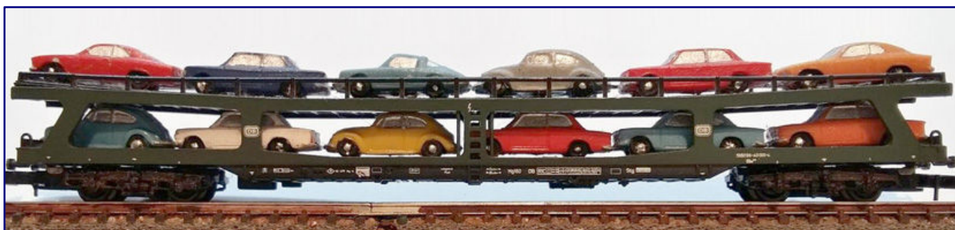
Two examples of DDm car transport wagons that can run on long-distance trains: up to twelve vehicles can be loaded on both floors of this double-decker wagon.
