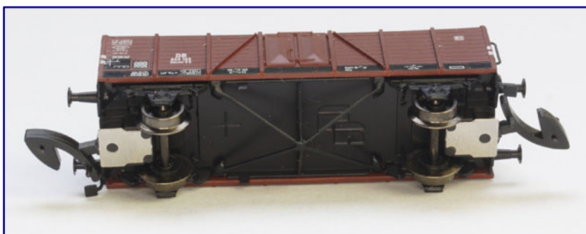
View of the wagon floor made of etched metal sheets with the spatial framework structure.
