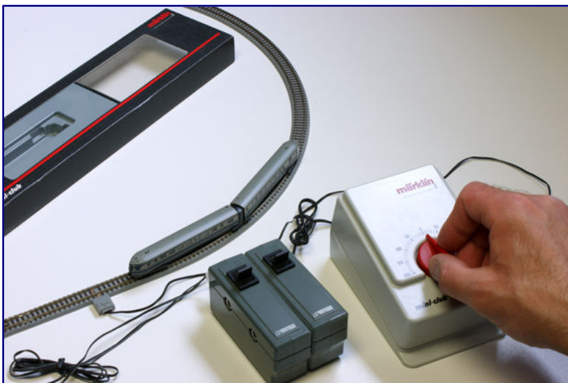
Before the conversion, there is still an analogue test run: the train should run perfectly, because digitisation does not cure mechanical problems!
