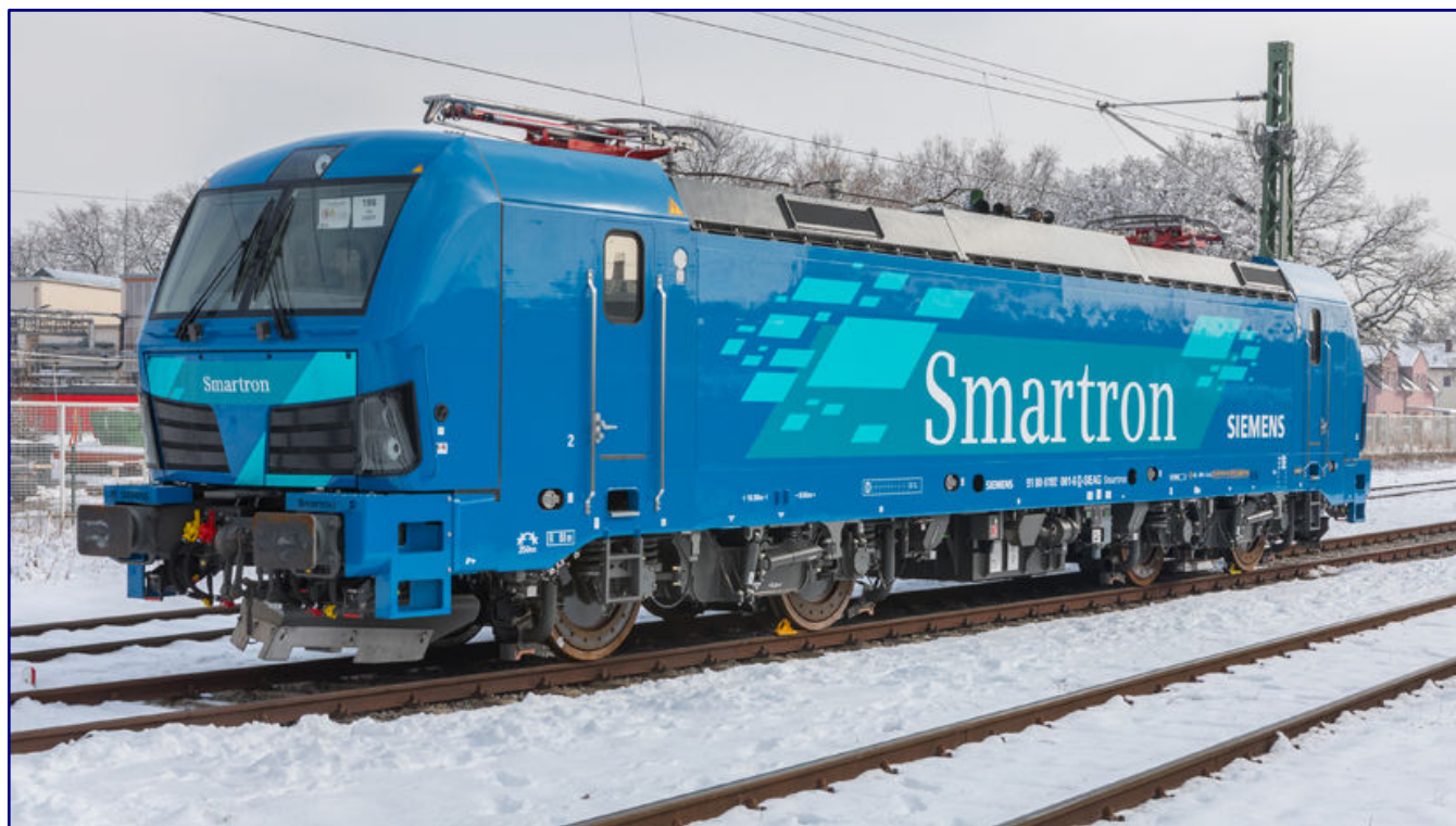
The name "Smartron", introduced in 2018, originally concealed a pre-configured AC locomotive for 15 kV 16.7 Hz with 5.6 MW power, listed in Germany as series 192. Due to demand, the range has since been extended to Romania and Bulgaria, and Italy could soon follow. Photo: Siemens Mobility (Siemens-Pressfoto)
