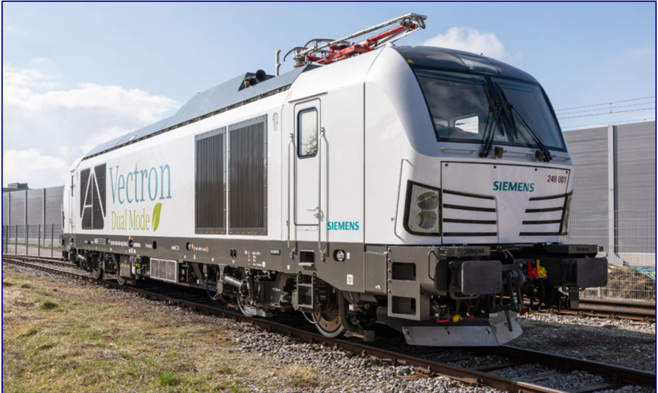
The latest addition to the Siemens platform is the Vectron DM (Dual Mode) for operation on an overhead line or with the aid of a diesel engine on sidings and feeder tracks. 248 001 was the first locomotive to be presented with this solution. Photo: Siemens Mobility (Siemens-Pressfoto)
