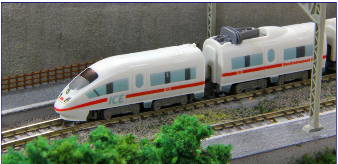
Rokuhan has high hopes for the greatly shortened and simplified vehicles of the Shorty series. Their rigid bogies can be exchanged for rolling, as well as powered bogie bases, and, thus, put into service. Photo: Rokuhan
