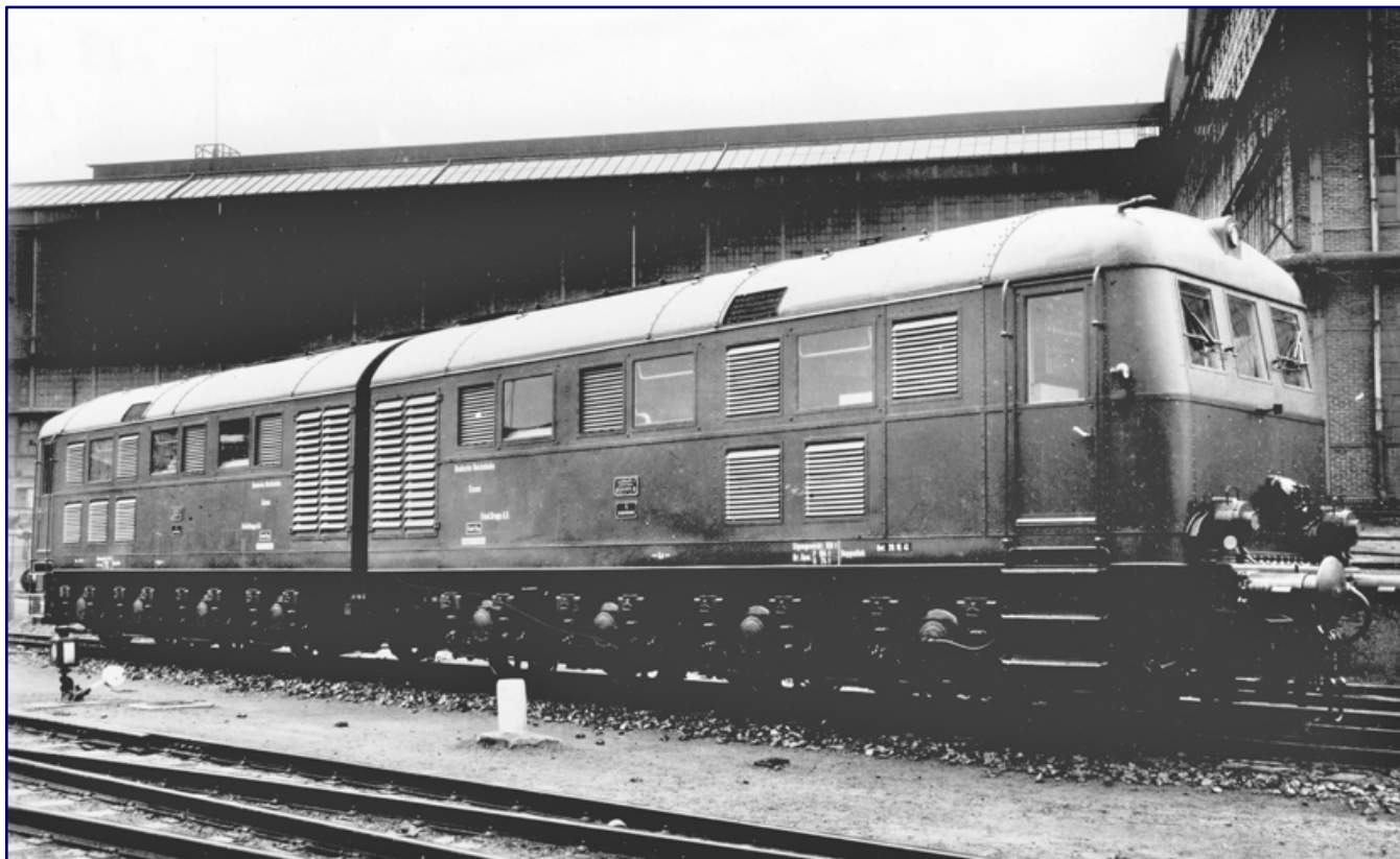
On 20 October 1941, the Wehrmacht locomotive D 311 a/b is ready for acceptance at the manufacturer Krupp in Essen. The blackout attachments on the lower locomotive lanterns bear witness to the Second World War. Only a few photographs from before 1945 show how the Wehrmacht locomotives were labelled when they were delivered. Photo: Krupp works photo, Eisenbahnstiftung
