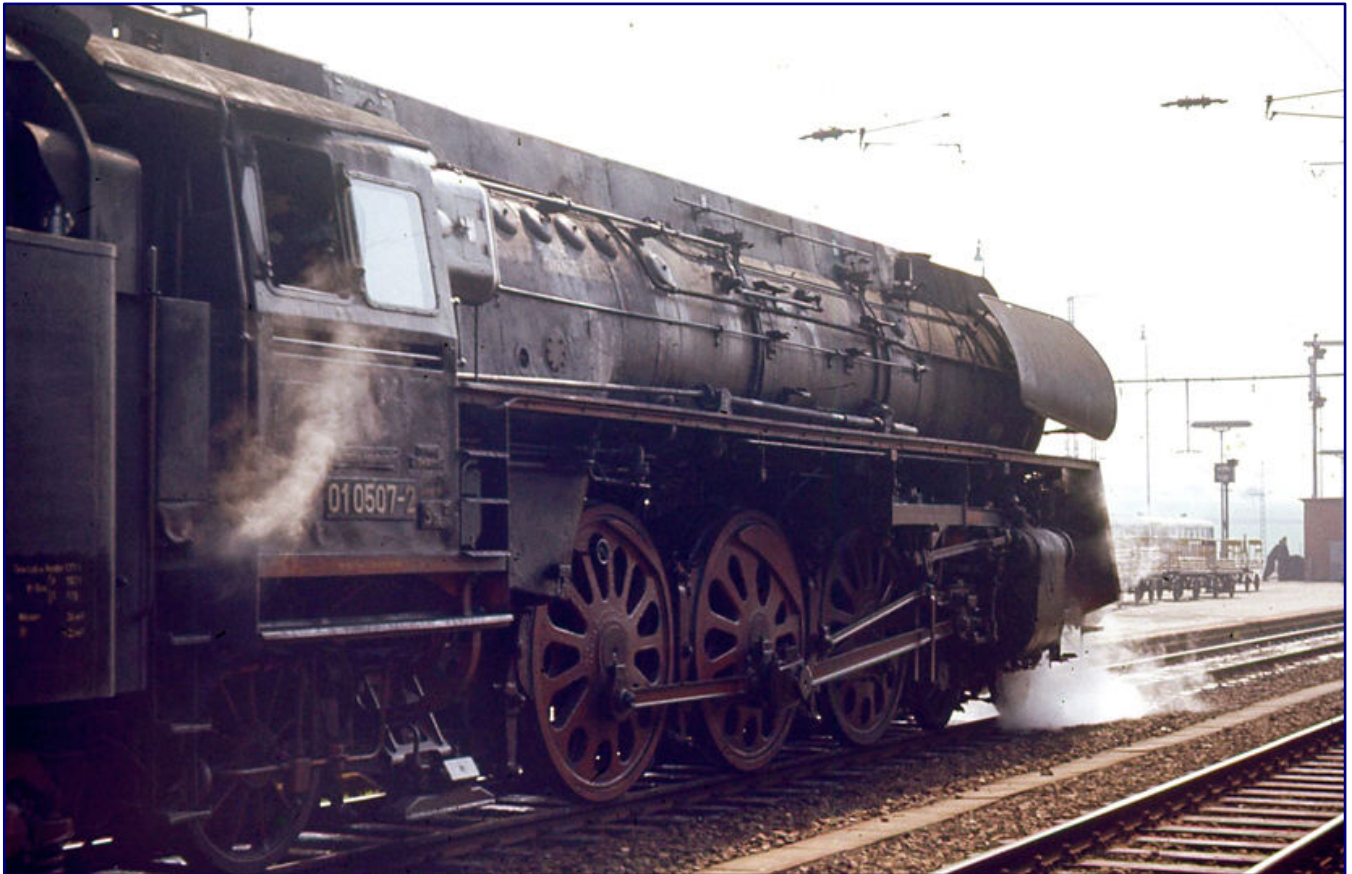
In 1972, the Reko locomotives also came to the territory of the DB in transit traffic. This is how 01 0507-2, still equipped with Boxpok wheels, could be photographed in Bebra. Photo: 8474tim (CC-BY-SA-3.0)
