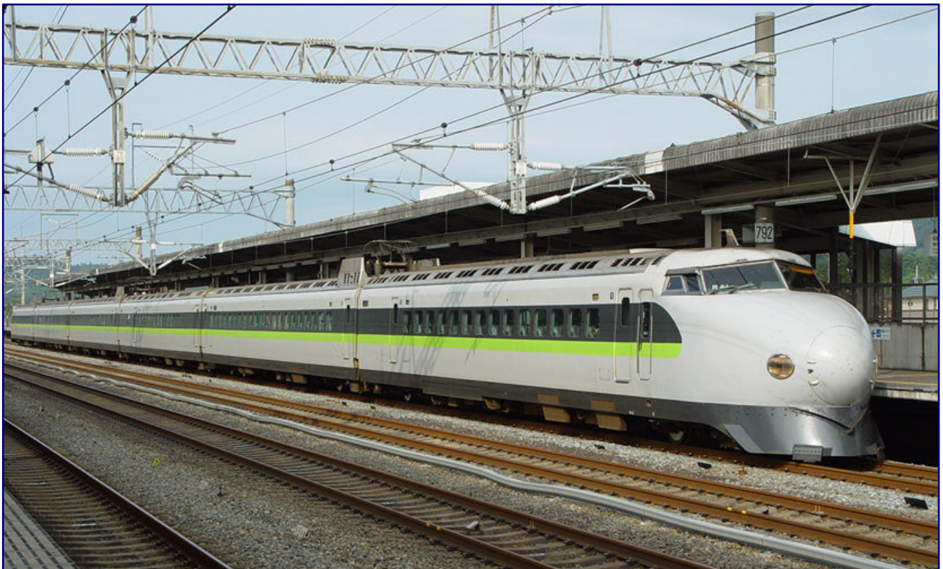
As Kodama 635, this six-car unit is travelling in new, very attractive colours as it passes in front of the photographer's lens in Higashi-Hiroshima on the San'yō line. The train runs from Shin-Osaka to Hakata. The train shows wind deflectors next to the pantographs, and the smaller side windows described in the text, which were temporarily installed to save costs. Photo: © DAJF / Wikimedia Commons / CC BY-SA 3.0 & GFDL
